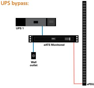
eATS Monitored can be used as a bypass to perform UPS maintenance without losing power to critical applications
