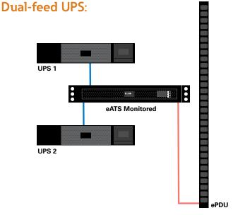
eATS Monitored manages input from a pair of UPSs to create a redundant environment ensuring system uptime
