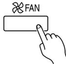
Press the fan control button to set the fan speed.
