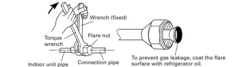
To prevent gas leakage, coat the flare surface with refrigerant oil.
