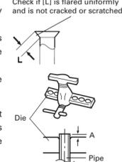
Insert the flare nut (always use the flare nut attached to the indoor and outdoor units respectively) onto the pipe and perform the flare processing with a flare tool.
