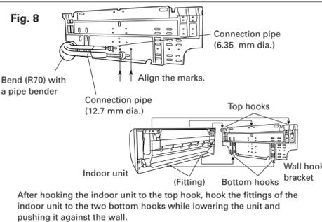
After hooking the indoor unit to the top hook, hook the fittings of the indoor unit to the two bottom hooks while lowering the unit and pushing it against the wall.
