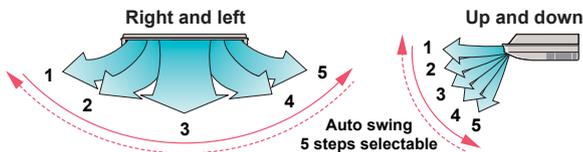
**Long distance airflow** Due to air blasting performance of maximum 18m, long-reach airflow is available for both cooling and heating operation.
