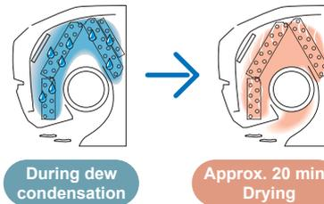
This model is equipped with an inner drying function. After the power is turned off, the dry operation starts inside the air conditioner. This prevents the growth of mold and bacterial inside the air conditioner.
