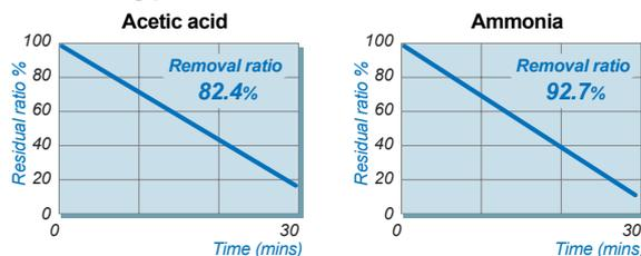
Test method: JEM1467 Test room: 1m<sup>3</sup>, acrylic sealed box
