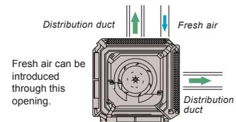
Conditioned air can be distributed by means of a distribution duct.
