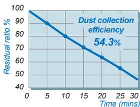
Test method: JEM 1417 Test room: 30m<sup>3</sup>, sealed room
