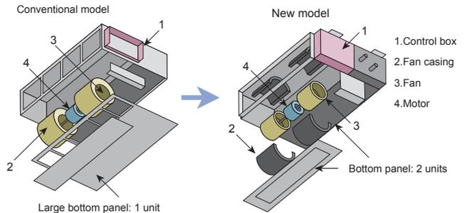
Structural improvement is attained by making the bottom panel two pieces, front and rear, and the internal fan casing is also made dismountable in two pieces, namely, upper and lower ones. The motor and fan maintenance and dismounting can be made easily by removing the rear panel and lower part of the casing with the main chassis installed.
