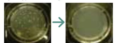
The undiluted solution of the specimen was made the specimen fluid and suspensoid 0.1ml (approximately 10<sup>7</sup>CFU/ml) of the test bacteria was inoculated.
