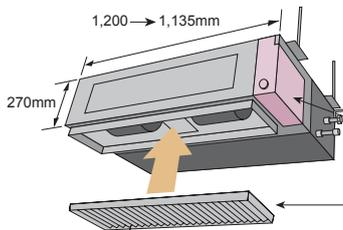
In the case of bottom suction type, as seen from lower rear part. In addition to the slim height of 270 mm which is our sales point, further compactification is attained by reducing 65mm from the width with the flanking controlbox embedded inside the chassis.
