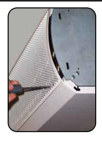
When making electrical connections first remove the safety cover plates over the electrical supply terminals. On 2m electric air curtains the safety cover plates are located towards the centre of the air curtain (See Insert).
