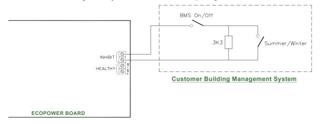
• A **HEALTHY** two screw terminal is included on the board for a fault signal indication if the electric elements overheat cut-out has operated. A healthy system provides a 24V DC signal at the terminals compared to an overheat fault which provides OV DC.
