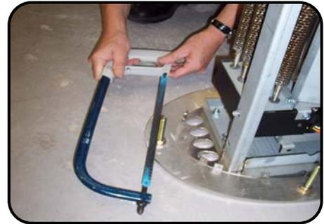
Remove only one M10 nut and refit and secure bolt with a stainless steel M10 dome nut supplied. Repeat for each of the other three projecting bolts one at a time.
