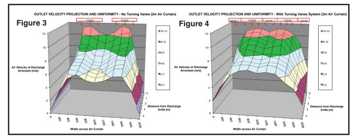
The 3D surface charts show this for a 2m Designer PHV air curtain where the low velocity areas shown at the ends and the middle in figure 3 are "filled-in" by the turning vane system as shown in figure 4.
