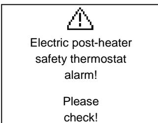
Safety thermostat electric heater intervention alarm. The thermostat intervenes at 115°C and is with manual re-arm. The unit continues working.
