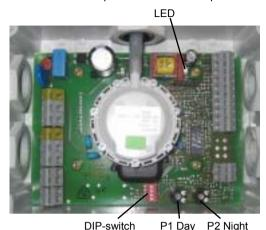
Via DIP-switch, the closed-loop parameters can be set. Those DIP-switches are numbered 1-4 beginning at the PCB rim. The view given above shows the DIP switch switched on to the left and switched off to the right.
