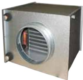
**CWK**, cold water-cooling battery for circular ducts. Casing of galvanised sheet steel with copper tubes and aluminium fins. Inspection covers for easy cleaning and maintenance.
