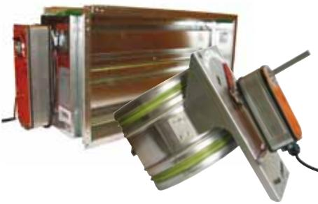
Shutter damper EFD is a shut-off damper suitable for Topvex. The damper is provided with 24V AC motors with spring-return actuators. EFD are made in leakage performance class 3 according to EN 1751:1998 Annex C.2. Outdoor air dampers are used to prevent the hot water battery from freezing and also prevent cold air to chill down the building if the unit stops. EFD is connected to terminals in the electrical connection box.
