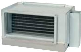
**PGK**, cold water-cooling battery for rectangular ducts. Casing of galvanised sheet steel with copper tubes and aluminium fins. Air vent and drain valve included. Condensation tray of stainless steel and condensate connection ( $R\frac{1}{2}''$ ). Max working pressure 1.6 MPa (16 bar). For water connection left or right.
