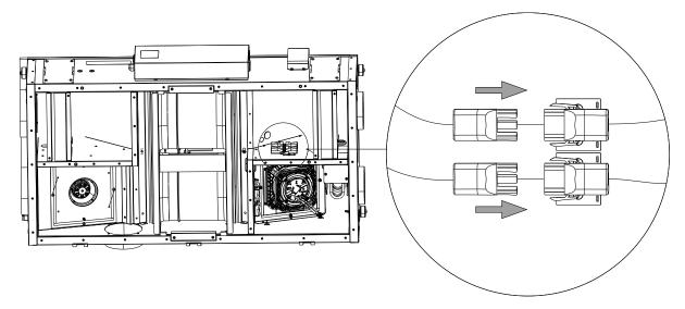
If the filter was removed in order to disconnect quick release connections, assemble all parts in reverse order: reconnect quick release connections (pos 4), mount filter (pos 3), place the bracket (pos 2) and tighten it with screws (pos 1).
