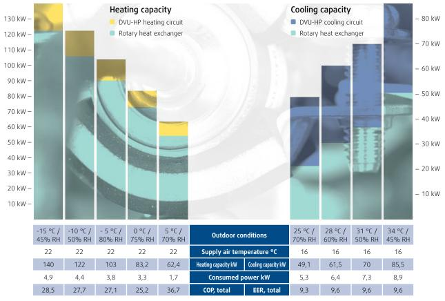
Performance example: DV 40 with 2,5 m³/s. Extract 22 °C/35% RH. Defrosting is not taken into account.
