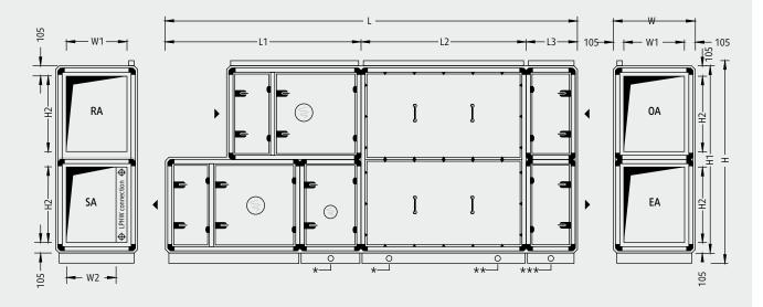
Important! Where a system is operated in parallel, the supply air and return air ducts of the two units have to be brought together.
