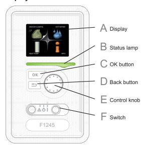
There is a display unit behind the heat pump door, which is used to communicate with F1245. Here you:
