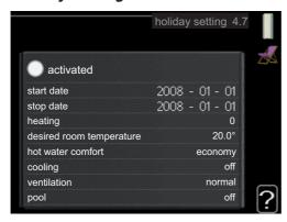
To reduce energy consumption during a holiday you can schedule a reduction in heating and hot water temperature. Cooling, ventilation and pool can also be scheduled if the functions are connected.
