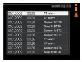
To facilitate fault-finding the heat pump operating status at alarm alerts is stored here. You can see information for the 10 most recent alarms.
