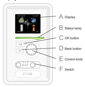
There is a display unit behind the heat pump door, which is used to communicate with F1145. Here you:
