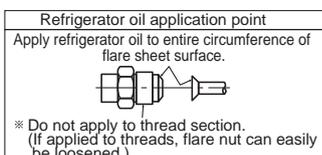
3) Securely tighten flare nut using torque wrench according to the table on the right.
