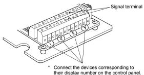
· Connect the centralized controller to the adapters as shown below.
