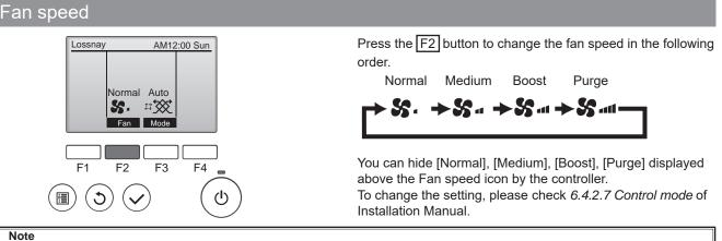
Base notch: The [Base notch] is the fan speed of standard for constant ventilation.
