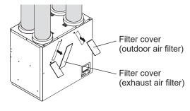
3) Gently draw out the outdoor air filter case and the exhaust air filter case.
