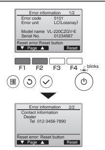
Error code, error unit, unit model name, and serial number will appear.
