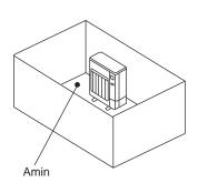
B) Install in a space with a depression height of [ 0.125 [m]
