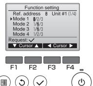
(5) When the settings are completed, press the  $\checkmark$  button to send the setting data from the remote controller to the indoor units.
