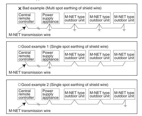
If there are more than 2 earthing spots on the shield wire, noise may enter into the shield wire because the earth wire and shield wire form 1 circuit and the electric potential difference occurs due to the impedance difference among earthing spots. In case of single spot earthing, noise does not enter into the shield wire because the earth wire and shield wire do not form 1 circuit.
