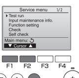
② Select "Test run" with the F1 or F2 button, and press the 🔾 button.
