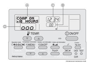
(1) Press the TEST button for 3 seconds to switch to maintenance mode.
