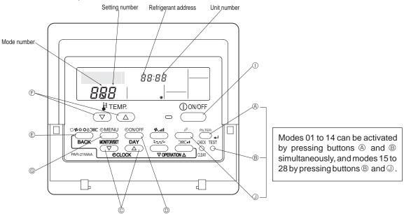
Selecting functions using the wired remote controller
