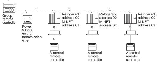
It would be acceptable if M-NET wire (non-polar, 2-cores) is arranged in addition to the wiring for A-control.
