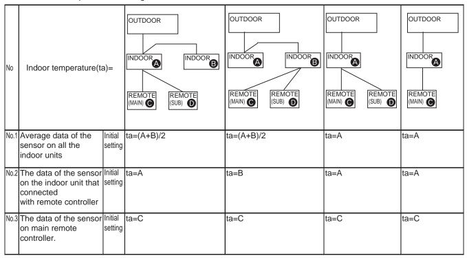
(2) Functions available when setting the unit number to 01-02 or AL (07 in case of wireless remote controller) Refer to the service manual that comes with each indoor unit.
