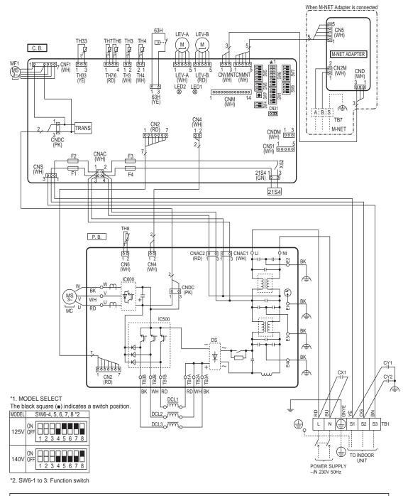
Never splice the power cable or the indoor-outdoor connection cable, otherwise it may result in a smoke, a fire or communication failure.
