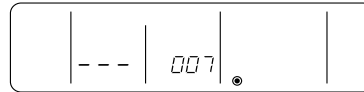
LOSSNAY can be searched in the same manner by bringing up the LOSSNAY address in the Interlocked unit address display window.
