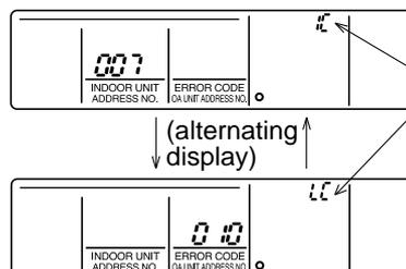
These alternating IC or LC displays will appear when entry is completed normally.
