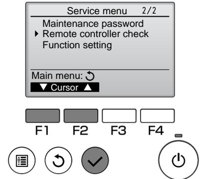
② Select "Remote controller check" from the Service menu, and press the
