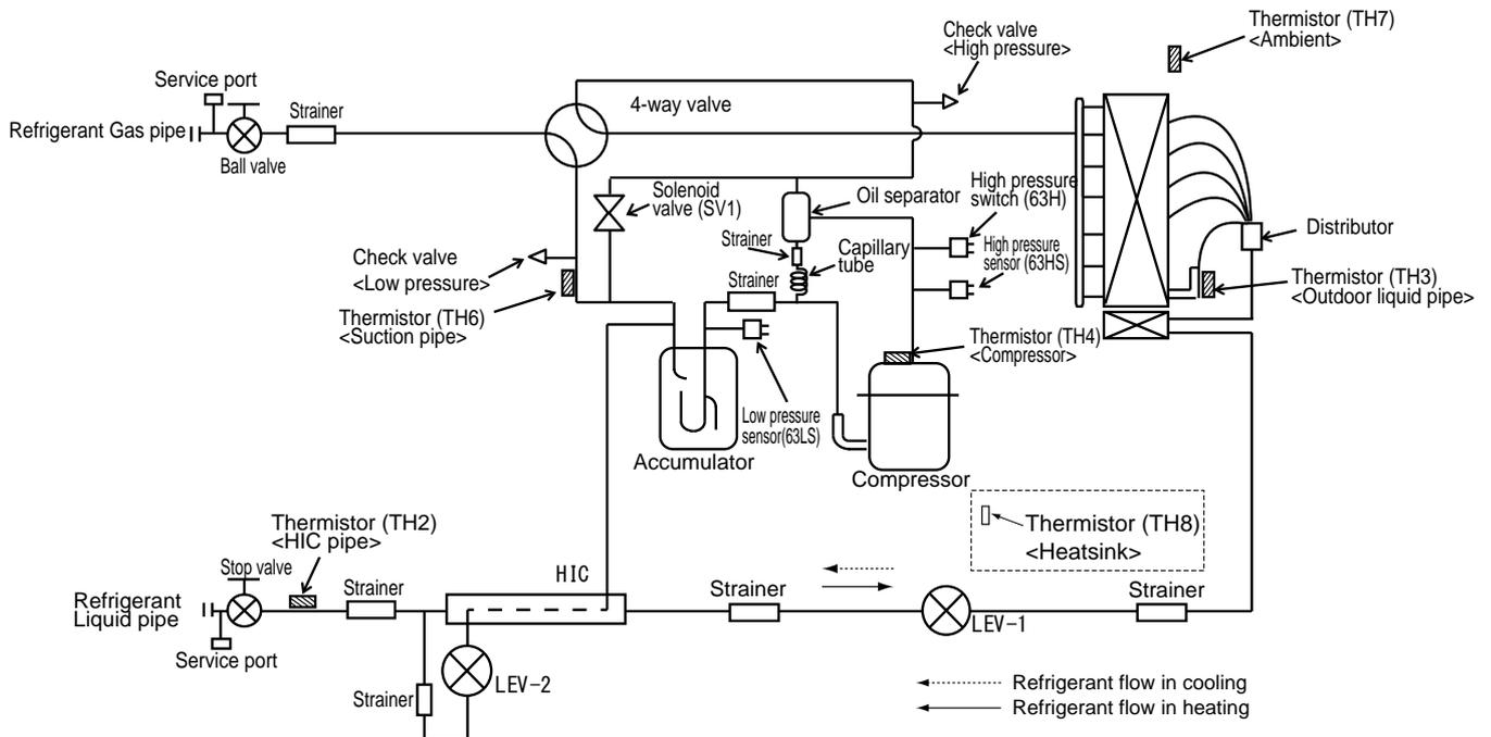
Capillary tube for oil separator :  $\phi 2.5 \times \phi 0.8 \times L1000$
