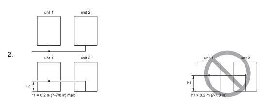
The NG example shows that oil accumulates into unit 1 while unit 2 is in operation, and unit 1 is stopped. Vertical pipe height (h) should be 0.2 m (7-7/8 in) or below.
