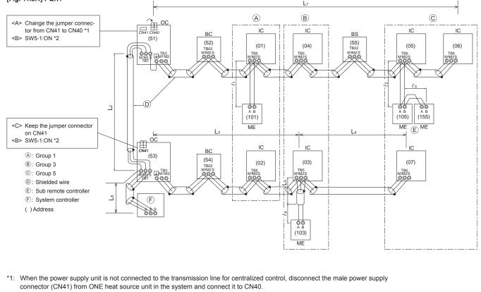
\*2: If a system controller is used, set SW5-1 on all of the heat source units to ON.
