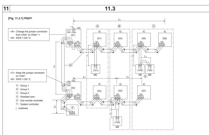
\*1: When the power supply unit is not connected to the transmission line for centralized control, disconnect the male power supply connector (CN41) from ONE heat source unit in the system and connect it to CN40.
