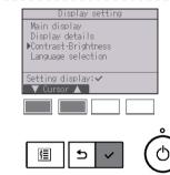
Move the cursor to "Contrast•Brightness" with the F1 or F2 button, and press the <u>SELECT</u> button.
