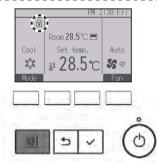
will appear on the Main display in the Full mode when the operation lock function setting is enabled.
