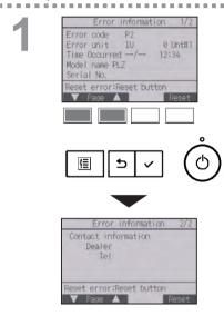
Error code, error unit, refrigerant address, unit model name, date and time on which an error occurred, and serial number will appear.
