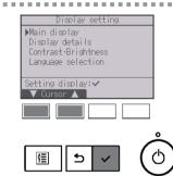
Move the cursor to "Main display" with the F1 or F2 button, and press the SELECT button.
