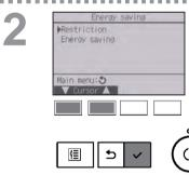
Move the cursor to "Restriction" with the F1 or F2 button, and press the SELECT button.
