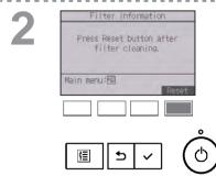
Press the F4 button to reset filter sign. Refer to the indoor unit Instructions Manual for how to clean the filter.
