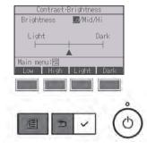
Adjust the brightness with the F1 or F2 button. Adjust the contrast with the F3 or F4 button, and press the MENU or RETURN button.
