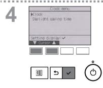
Move the cursor to "Clock" with the F1 or F2 button, and press the SELECT button.
