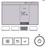
Each pressing of the F3 button cycles through the following ventilation settings.
