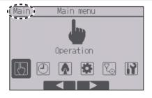
The following settings cannot be made from the sub remote controller. Make these settings from the main remote controller. "Main" is displayed in the title of the Main menu on the main remote controller. Timer (On/Off timer, Auto-Off timer, Weekly timer, Night setback, OU silent mode) Energy saving (Auto return, Schedule)
