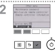
Move the cursor to "Initialize remote controller" with the F1 or F2 button, and press the SELECT button.
