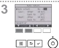
The screen to make the settings for the automatic return to the preset temperature will appear.
