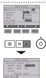
The screen to make the settings for the operation lock function will appear.
