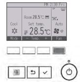
Each pressing of the  $\boxed{F4}$  button cycles through the following fan speeds.
