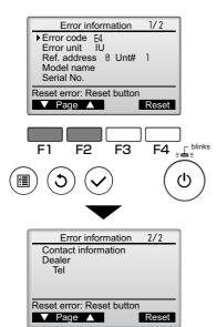
Error code, error unit, refrigerant address, unit model name, and serial number will appear.
