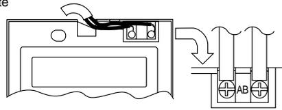
To connect the remote control cord, peel 6mm of coating.
