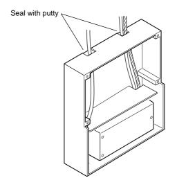
(13) Install the controller inside the Mounting attachment A type with the four M4 rounded screws (supplied).
