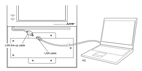
Remove the cover of Mounting attachment A type to use the LAN link-up cable. Refer to section 1.(1) in (6.|Installation) for how to remove the cover.
