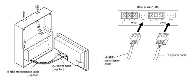
DC power line and M-NET transmission cable are connected using a connector as shown figure below. Connectable to the connector using the cable that is supplied.
