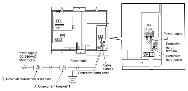
\*1 When using a fuse, use it in combination with a main switch (Rated current: 3A).
