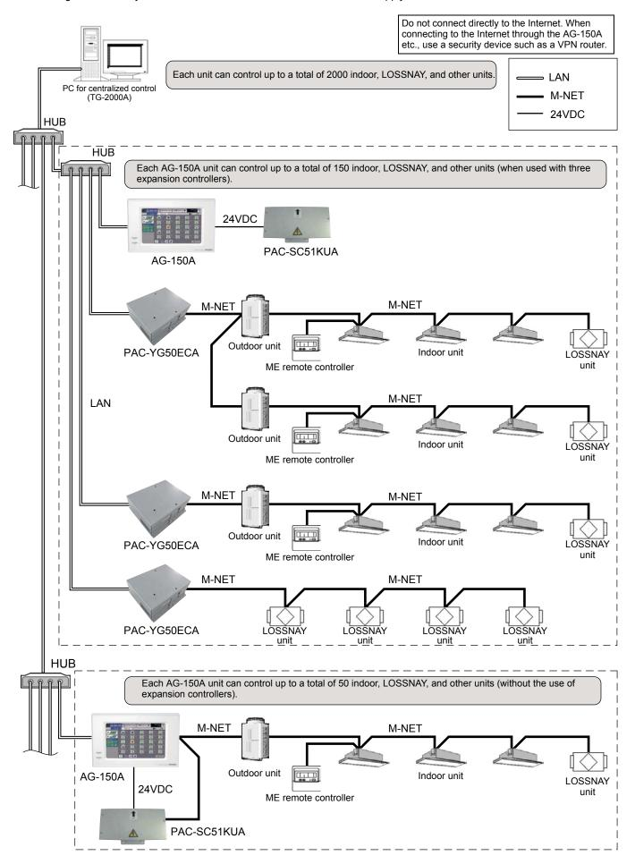
• Address setting for various devices: The same address cannot be used more than once within the same system of the expansion controller (PAC-YG50ECA). (K-control units and K-control remote control addresses are excluded.)
