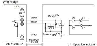
Use relays that meet the following specifications for Z1 and Z2. Operation coil
