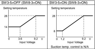
\*When the setting temperature in heating mode is 17 or less, the discharge air temperatutre can be unstable.
