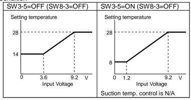
\*When the setting temperature in heating mode is 17 or less the discharge air temperature can be unstable.
