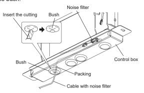
5) Install the insulating sheet on the control box. Insert the control box to the unit, attach two screws. (Don't forget to place the insulating sheet) Bind the cable with noise filter with a cable strap (supplied with the unit) and attach it under the unit. (It is recommended to install it with flexibility so that it will not be loaded from the outside.)
