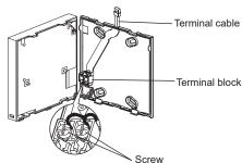
2) Connect the remote controller cable (field supplied) to the terminal block on the bottom case.
