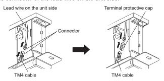
3) Connect the connector of the accessory cable with noise filter to the TM4 cable.
