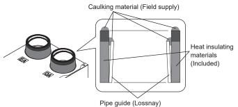
3) Place the Silencer box while aligning the position of the connection ports at the bottom of the Silencer box with the pipe guides of the Lossnay unit. Make sure that the under fix piece of the Silencer box touches the wall mount hook top of the Lossnay unit.
