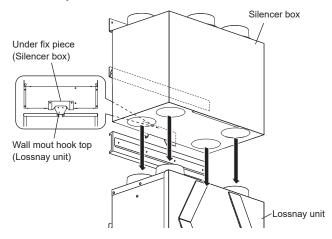
4) Fix the Silencer box with the two screws.
