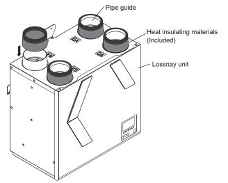
2) Apply a good amount of a caulking material (liberally) to the pipe guides and heat insulating materials. Insufficient application may cause water leakage and air leakage.
