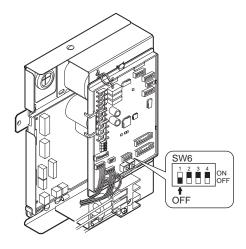
(3) Insert the connector of the air duct switching damper connection cord into the PCB connector [CN7] of Lossnay.
