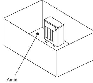
B) Install in a space with a depression height of  $\leq 0.125$  [m].
