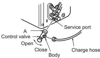
When attaching the control valve to the service port, valve core may deform or loosen if excess pressure is applied. This may cause gas leak.
