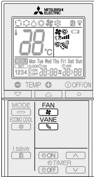
Press **FAN** to select fan speed. Each press changes fan speed in the following order:
