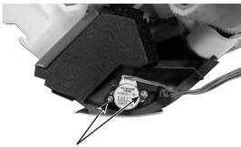
Screws of the vane motor
