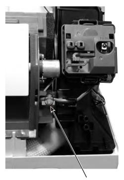
Fixing band of the vane motor wire
