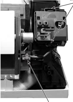
Fixing band of the vane motor wire
