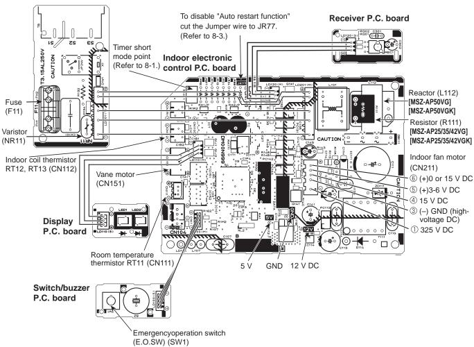
\*\* Please replace the fuse after removing the indoor terminal P.C. board from the electrical box.
