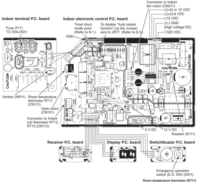
\*\* Please replace the fuse after removing the indoor terminal P.C. board from the electrical box.
