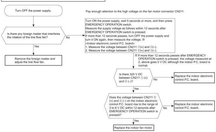
The indoor fan motor error has occurred, and the indoor fan repeats "12-second ON and 30-second OFF" 3 times, and then stops.
