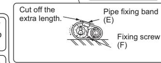
When the piping is to be attached to a wall containing metals (tin plated) or metal netting, use a chemically treated wooden piece 20 mm or thicker between the wall and the piping or wrap 7 to 8 turns of insulation vinyl tape around the piping.
