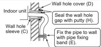
After the leak test, apply insulating material tightly so that there is no gap.
