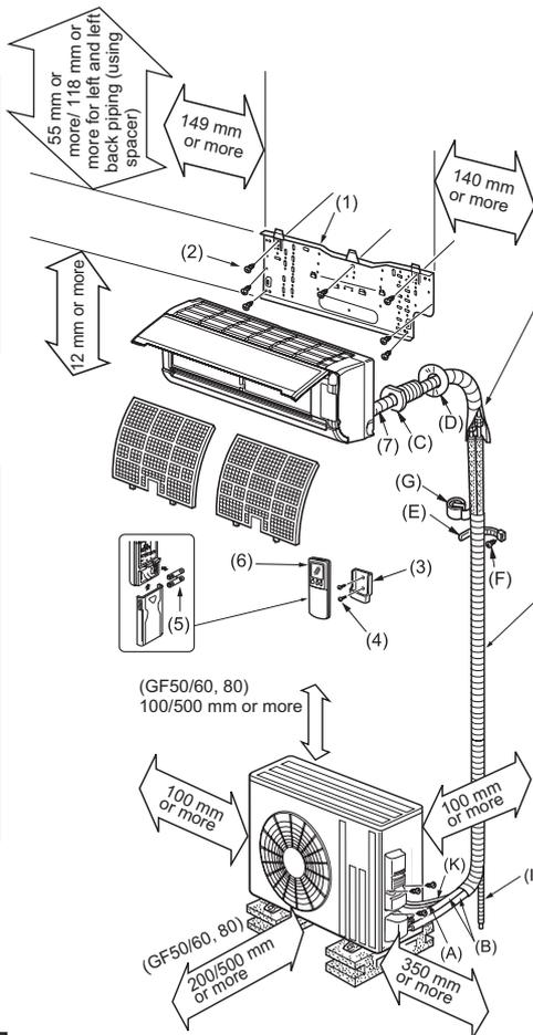
Be sure to use wall hole sleeve (C) to prevent indoor/outdoor connecting wire (A) from contacting metal parts in the wall and to prevent damage by rodents in case the wall is hollow.
