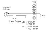
To use operation monitor output for a supply after-heater, turn SW2-8 ON, and use the supply fan operation monitor output with delayed operation. (Refer to function settings No. 57) For the heater, observe the cautions listed in 4.
