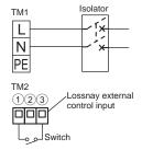
Start/stop the unit by a switch connected to TM2(1)(3). When turned the unit ON, it operates at fan speed 4 and automatic ventilation mode. Do not start/stop the unit by turning the power supply to the unit
