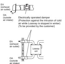
In a region where there is risk of freezing in winter, it is recommended to install an Electrically operated damper, or the like, in order to prevent the intrusion of (cold) outdoor air while Lossnay is stopped.
