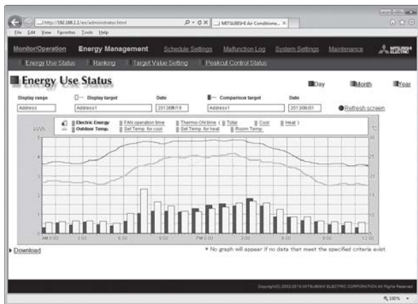
Energy Management monitor (Energy use status)
