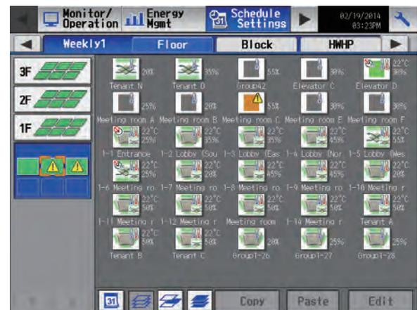
Note: The [HWHP] tab will appear when an HWHP (CAHV, CRHV) unit is connected.
