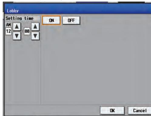
Note: When setting a schedule for a block or all groups, all operation modes are available for selection, but the available operation modes depend on the unit model. The units will not operate in the selected mode not supported by the units.
