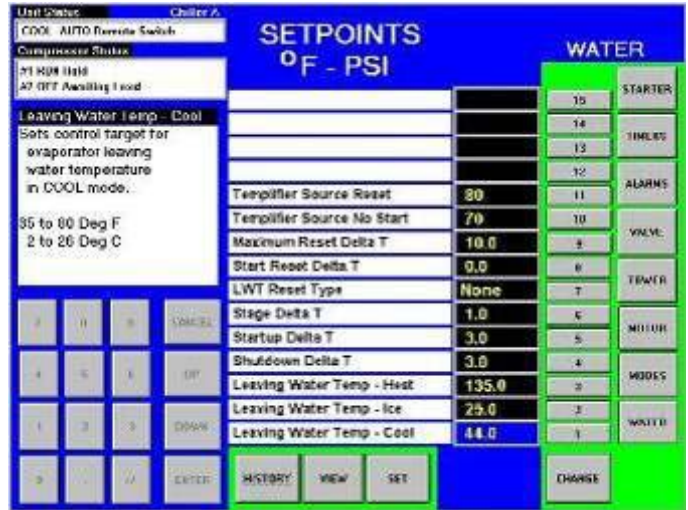
Figure 5, MicroTech II Setpoints Screen
