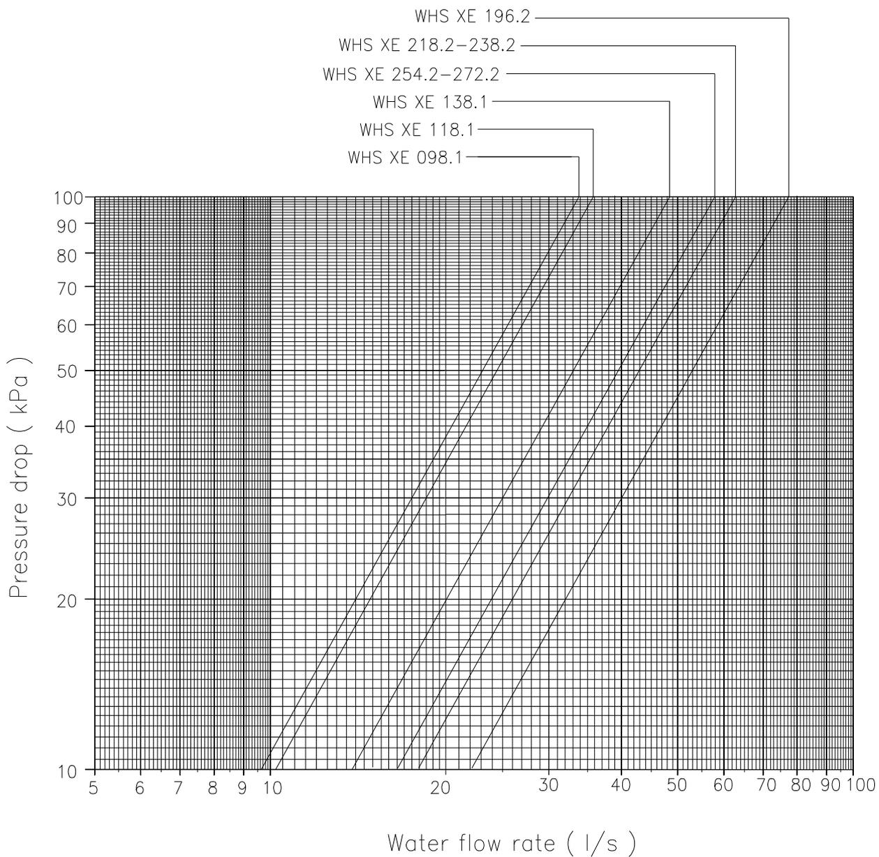
**Note:** in case of pressure drop higher than 100 kPa, it is necessary to contact the factory.
