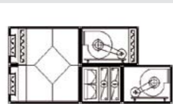
2. Horizontal with return and supply fan
