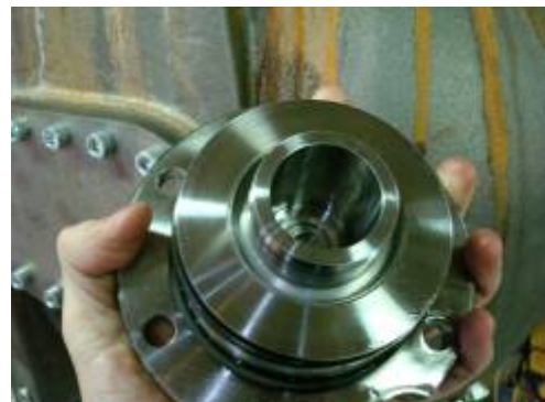
Removal of the filter housing cover
