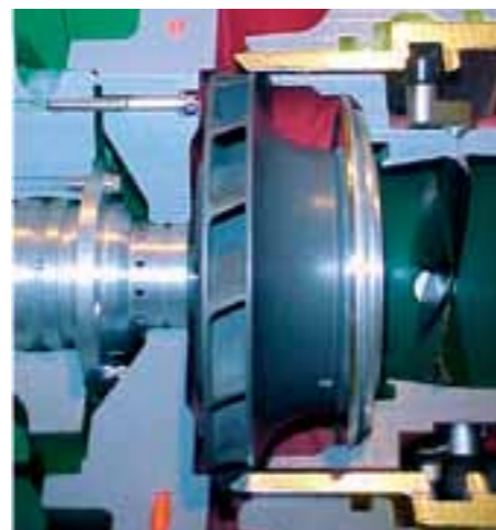
Moveable diffuser closing off impeller discharge area
