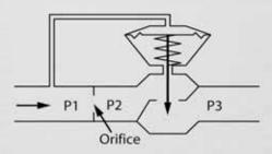
For the FlowCon A/AB/ABV, the principle of operation is shown above and the principle of construction is shown to the right. P1 and P3 are system pressures, P1÷P3 is the total pressure drop across the valve. P2 is set by the diaphragm acting in reaction to P1 in the upper diaphragm chamber. Interacting with the spring, P1÷P2 remains constant, keeping a constant  $\Delta P$  across the orifice areas. The result is a constant flow rate through the valve, independent of pressure fluctuations.
