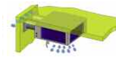
HPS in free cooling mode: use of external fresh air to maximise the energy saving
