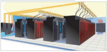
The Liebert XDV works extremely well with the "hot aisle-cold aisle" approach.
